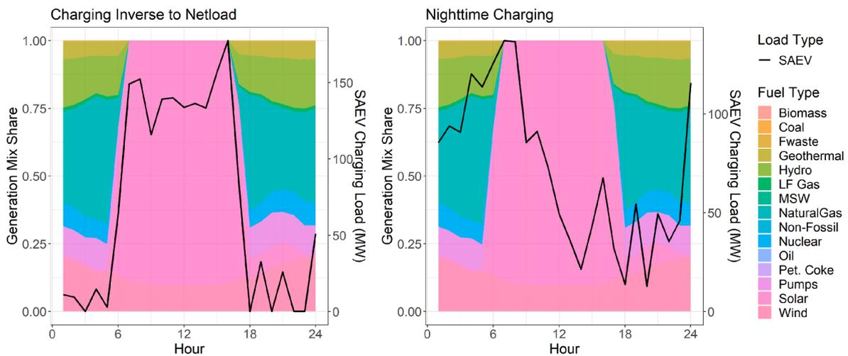
Fig. 5. Hourly generation mix in California and SAEV charging load of different charging strategies, on a typical spring day of 2030, with medium SAEV adoption level, occupancy rate of 1 passenger, and without applying carbon tax.
