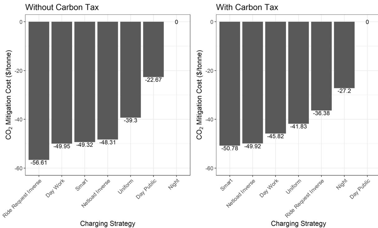
Fig. 11. Relative CO<sub>2</sub> mitigation cost by switching from the most carbon-intensive charging strategy to other charging strategies for SAEVs, under medium adoption level and occupancy rate of 1 passenger, 2030, California.
