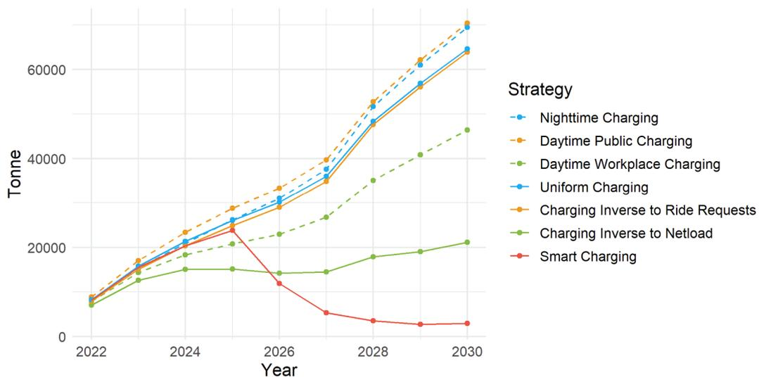
Fig. 6. Total annual CO<sub>2</sub> emission caused by SAEVs in California, under different charging strategies, with medium adoption level and occupancy rate of 1 passenger, without applying carbon tax.
