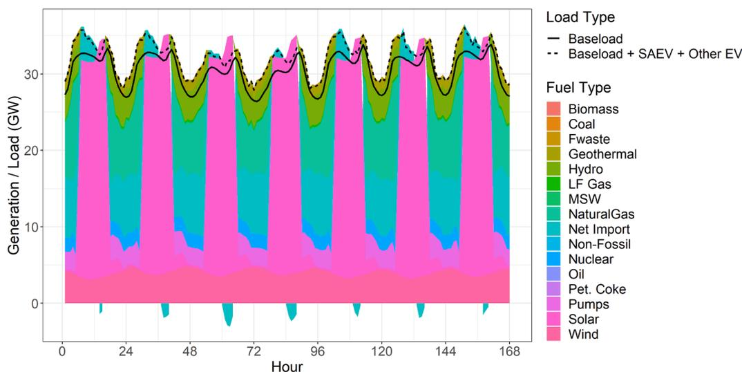
**Fig. 4.** Generation and load patterns of California in a typical spring week of 2030, with medium SAEV adoption level, occupancy rate of 1 passenger, and daytime workplace charging strategy, without applying carbon tax.
