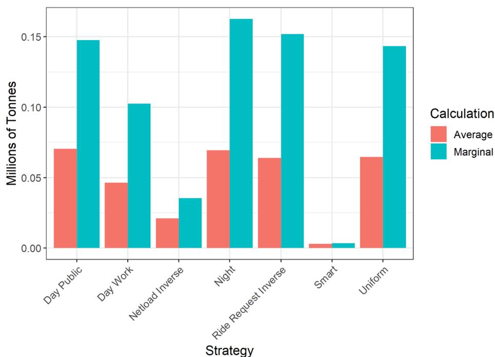
**Fig. A1.** Difference between average and marginal calculation of CO<sub>2</sub> emission, on the total annual CO<sub>2</sub> emission caused by SAEVs in California in 2030, with medium adoption level and occupancy rate of 1 passenger, without applying carbon tax.
