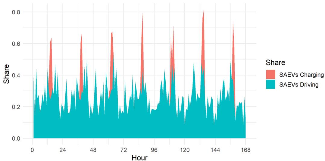
Fig. 12. Share of SAEVs charging and driving by hour, in 2030, with low adoption level of SAEVs, occupancy rate of 4 passengers, and smart charging strategy, without applying carbon tax.
