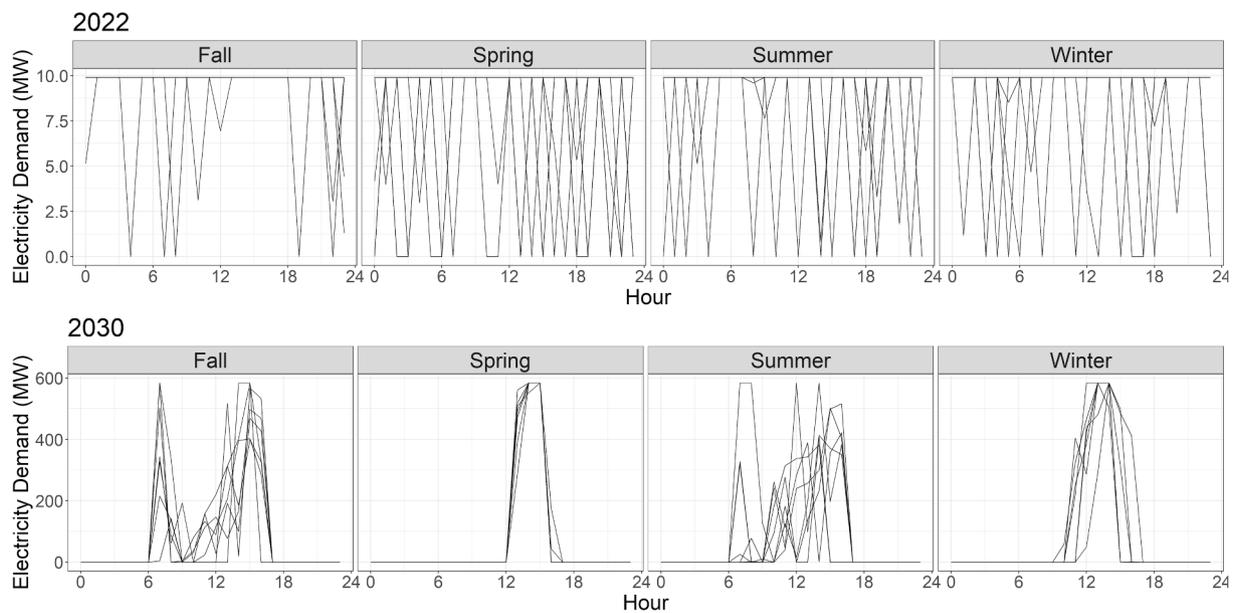
Fig. 7. Smart charging profiles in different seasons in 2022 and 2030, under medium adoption level and occupancy rate of 1 passenger, without applying carbon tax.
